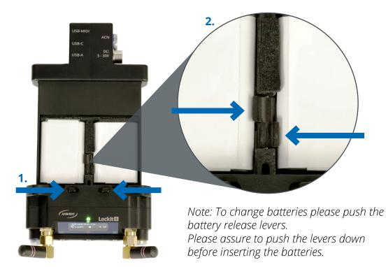
If the Lockit+ is switched off and power is applied, the LED will slowly blink red to indicate charging of the batteries. Fully charged, the LED will be lit permanently green.
